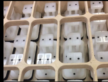
Male plugs to support suction cup pickup
